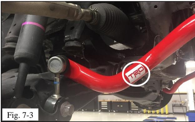
**⚠ CAUTION:** The TRD logo orientation should be confirmed for aesthetic purposes only (Fig. 7-3). DO NOT USE THE LOGO TO CONFIRM BAR ORIENTATION.
