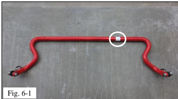
**STOP:** Make sure the stabilizer bar is set up in the correct orientation. Confirm that the “BOT” markings on the stopper rings are at the BOTTOM, the Part Number Label is on the RH side of the vehicle, and the arms of the bar point rearward (Fig. 6-1).
